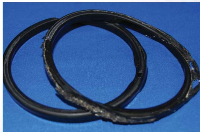
Piston u-seals showing evidence of pressure trap.
